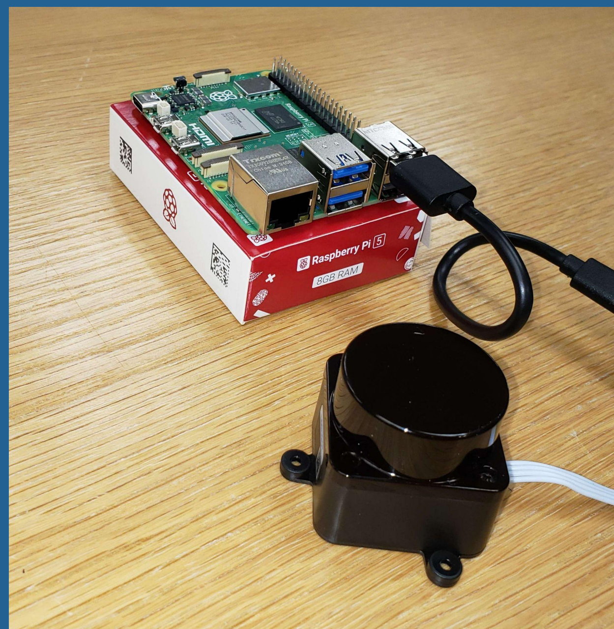
Photo of LiDAR and Raspberry Pi
