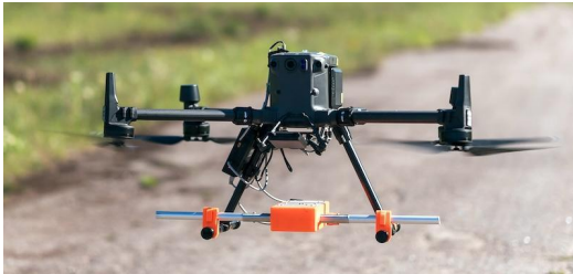
Drone-mounted GPR kit. Model shown can penetrate 12m below ground surface.
