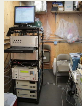
Elemental Hg 0 (Tekran 2537 Air Hg Analyzers)
