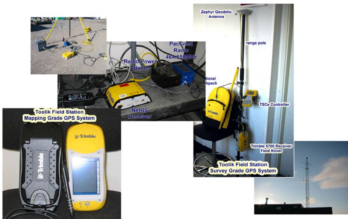
Figure 14. Toolik Field Station GPS equipment – Permanent Base Station, Mobile Base Station, Survey & Mapping Grade rover units, real-time corrected (RTK): accuracy ranges from 2m to 5mm depending on survey style.
