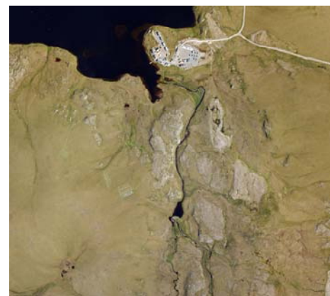
Figure 11. Mosaic of 24 frames from 2 flight lines covering the area around Toolik Lake. Photo mosaic is rectified with accuracy to ~2m in ground coordinates.
