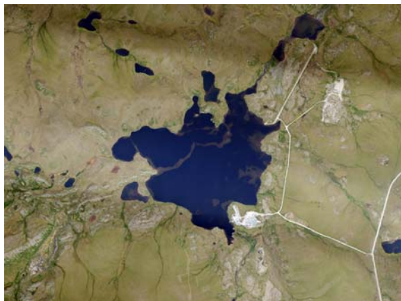
Figure 11. Mosaic of 24 frames from 2 flight lines covering the area around Toolik Lake. Photo mosaic is rectified with accuracy to ~2m in ground coordinates.
