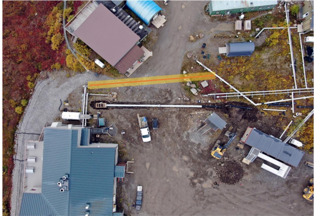
Highlighted Area shows Dining Facility waste line location that will be excavated and releveled for proper slope to the Central
