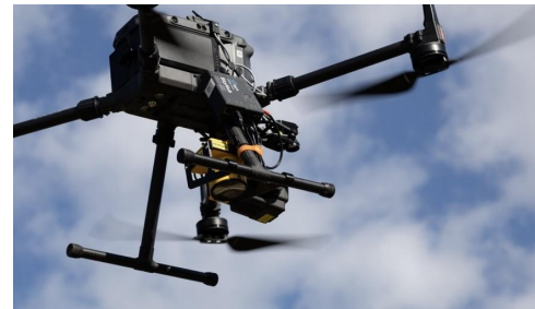
Drone-mounted methane sensor. Data available real-time and post-collection.
