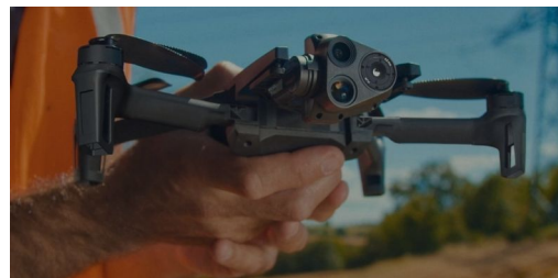
Thermal and RGB sensors integrated into small drone platform.
