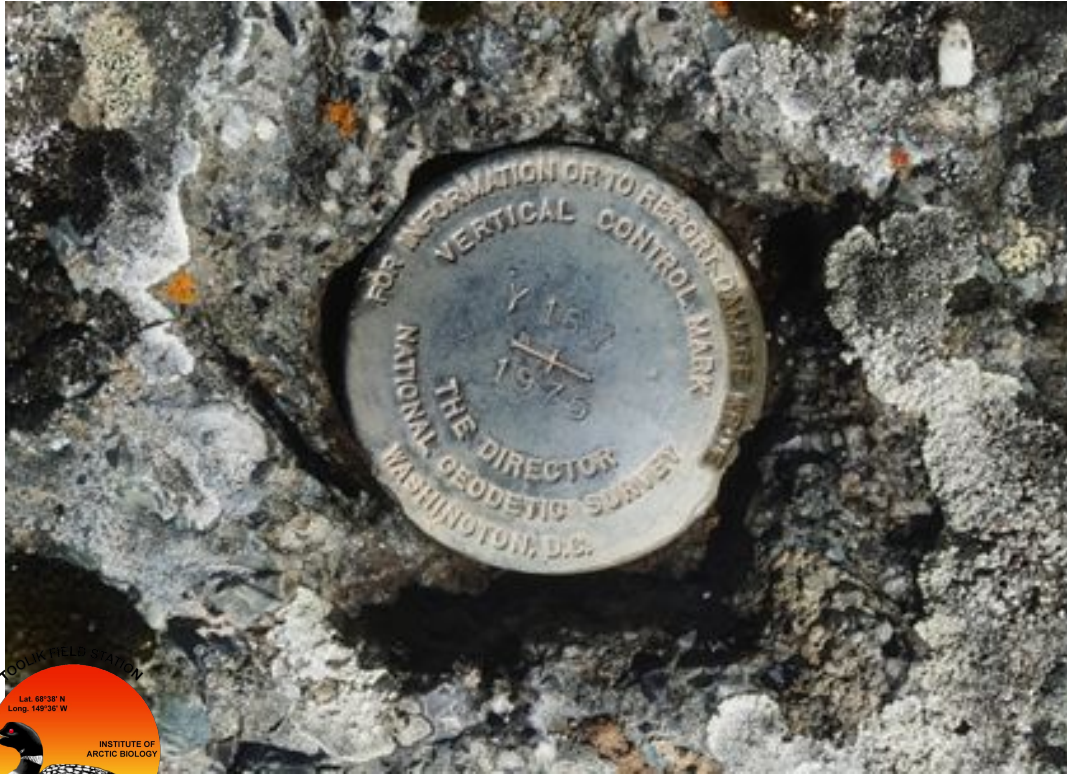
NGS benchmark embedded in a rock near Pump Station 4
