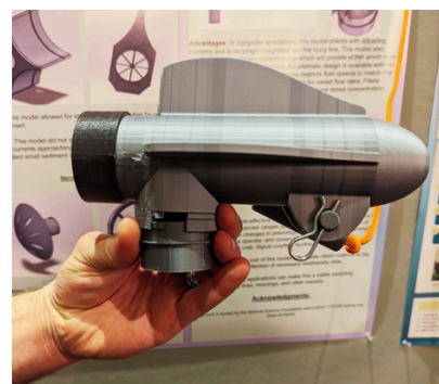
The passive eDNA sediment collection apparatus by Jessica Glass and the Glass Lab
