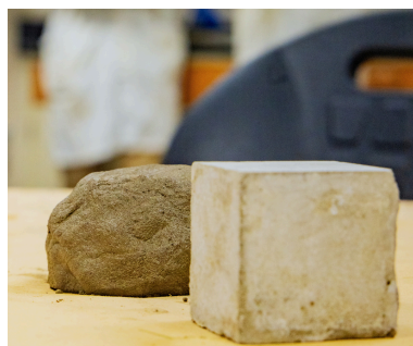
Alkali activated fly ash concrete by Nima Farzadnia and the Advanced construction and materials lab
