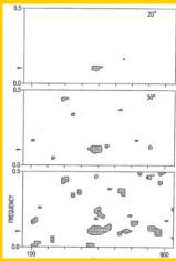
The detector's response over frequency and time for three acceptance angles, with dark areas showing detected signals and dotted lines marking the wave's temporal region.
