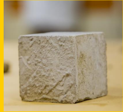
A concrete block made from fly ash.
