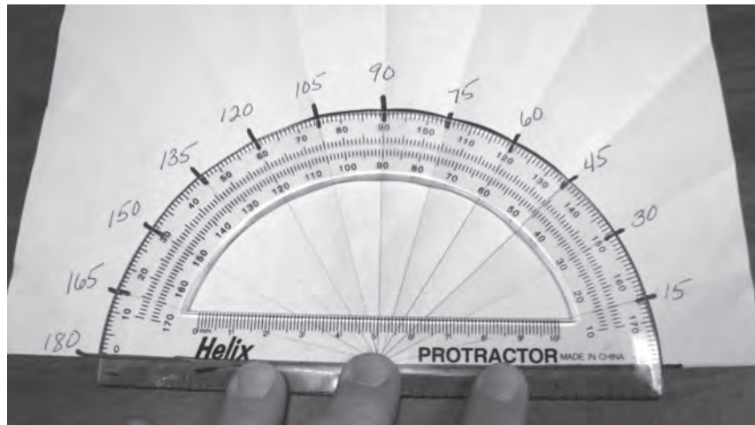
Fig. 6.2: Checking the personal protractor measurements against a commercial protractor.
