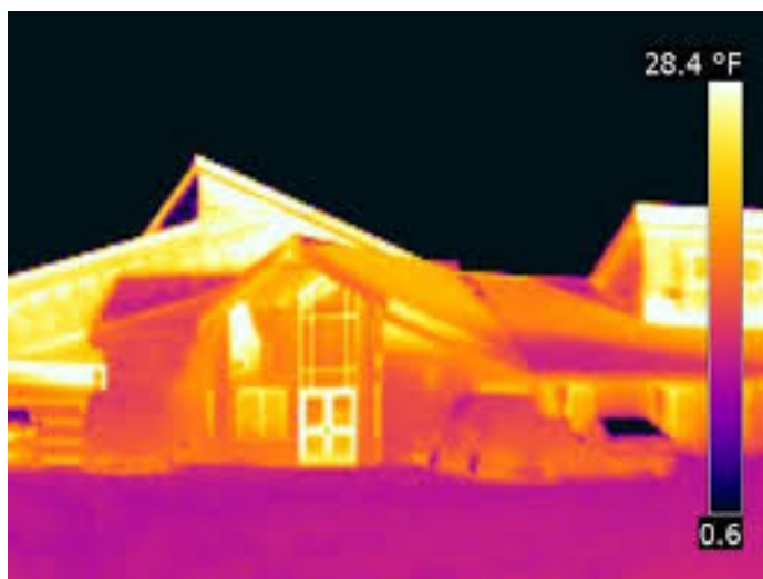
Fig. 3. Bristol Bay Campus heat loss test of campus building using infrared camera in Sustainable Energy course in Dillingham, AK.
