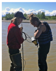
Cover photo by S. Hayes - Anna Liljedahl and Amanda Barker conducting field work near Delta, Alaska measuring water depth and flow rate in rivers.
