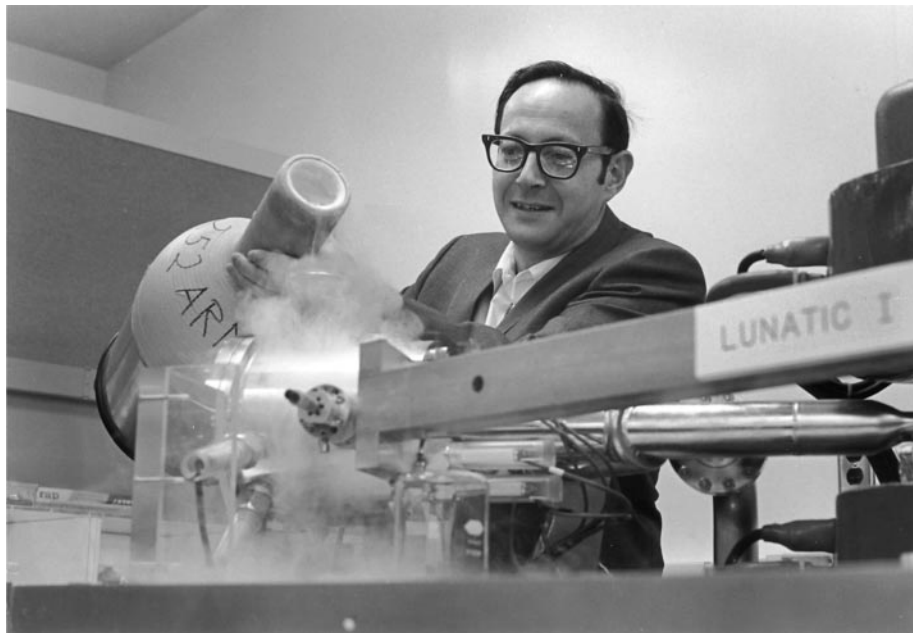
Figure 2 Filling liquid nitrogen in the ion source trap of the Lunatic I (circa 1970). Caltech archives.
