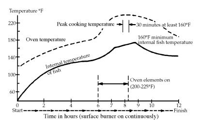
Figure 1. Typical internal fish temperature during smoking cycle.
