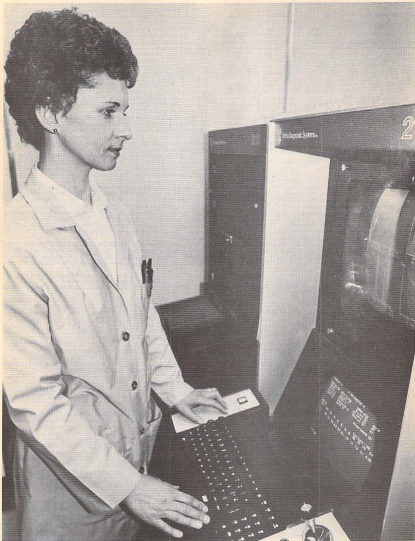
Betsy Robertson, research associate with the Institute of Marine Science, calibrates a flow cytometer, which is used for counting one-celled organisms in sea water.
