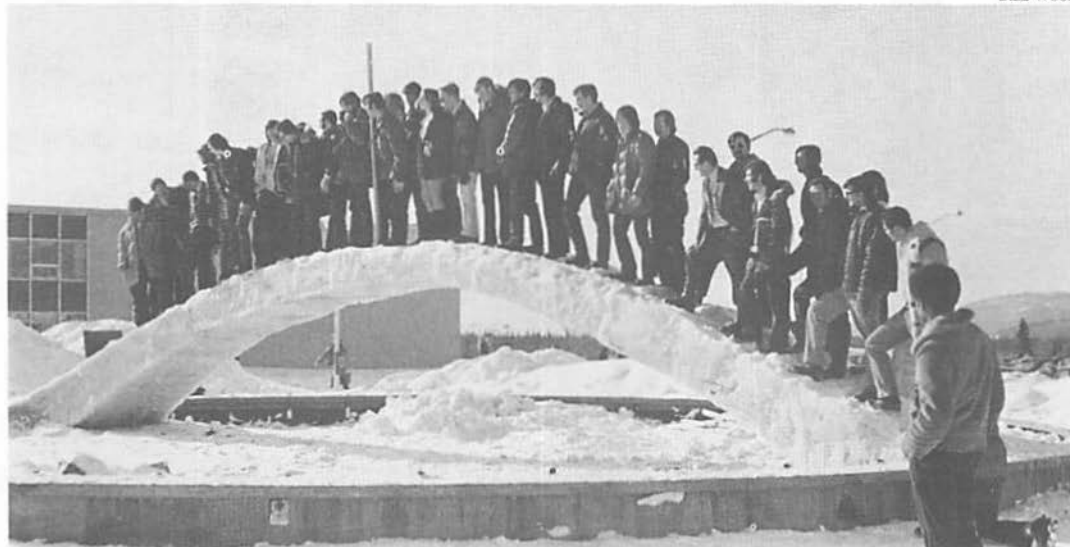
An ice arch constructed by civil engineering students proved capable of supporting a substantial load.
