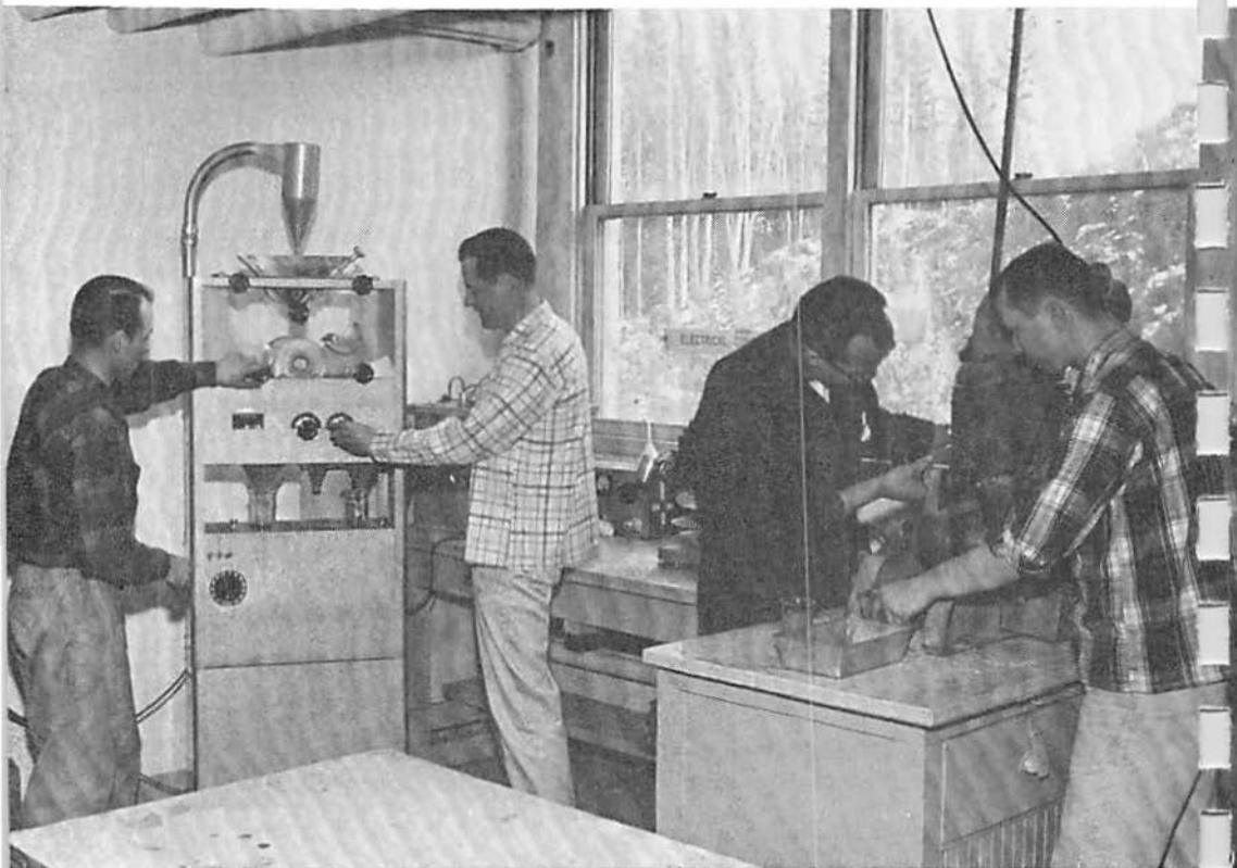
Geology students work with an electrostatic separator and an electromagnetic separator in the College of Earth Sciences and Mineral Industry.
