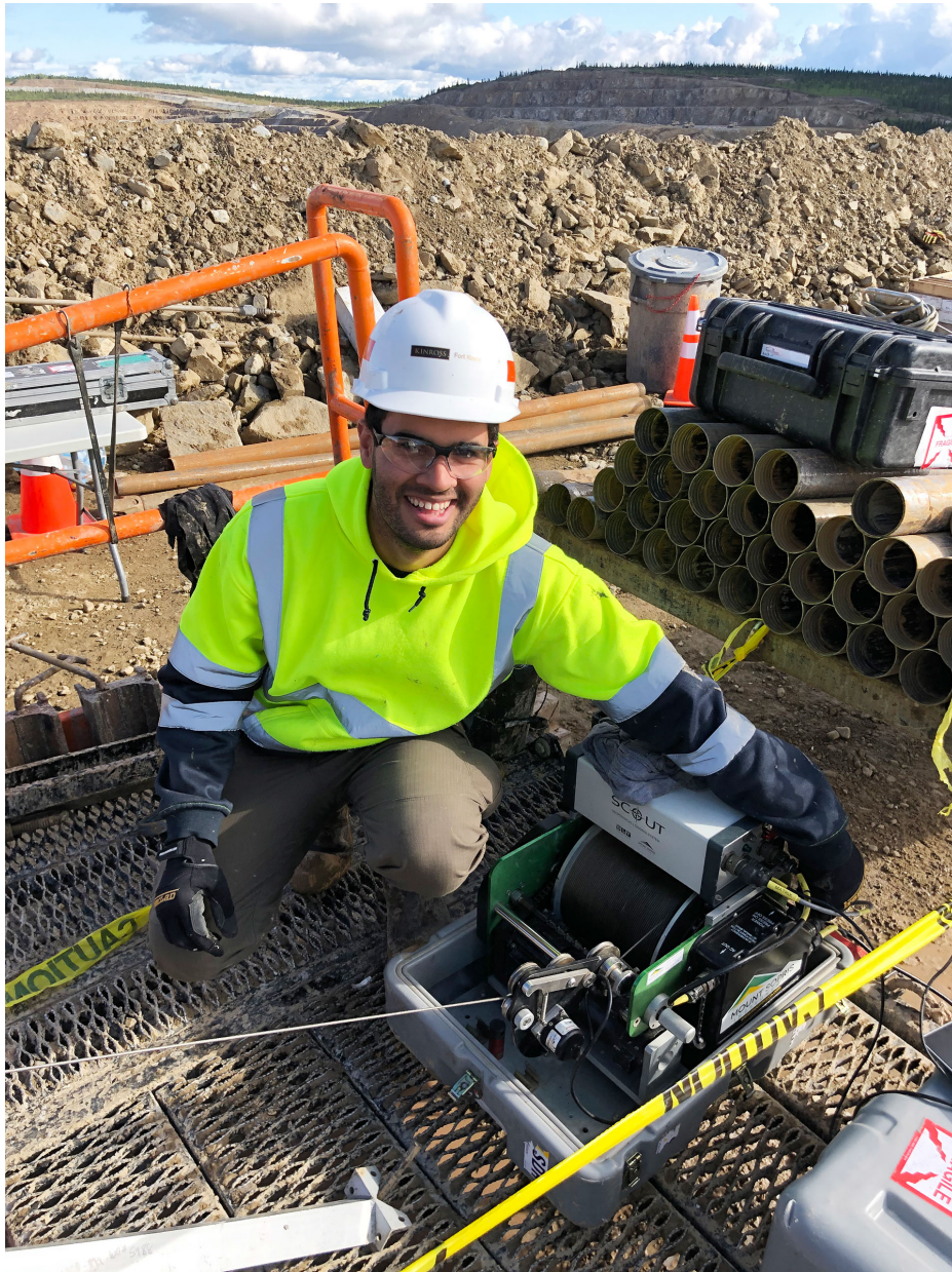
Juan Avila conducts a drill hole survey with an acoustic televiewer during a summer 2020 internship at the Kinross Fort Knox mine north of Fairbanks.
