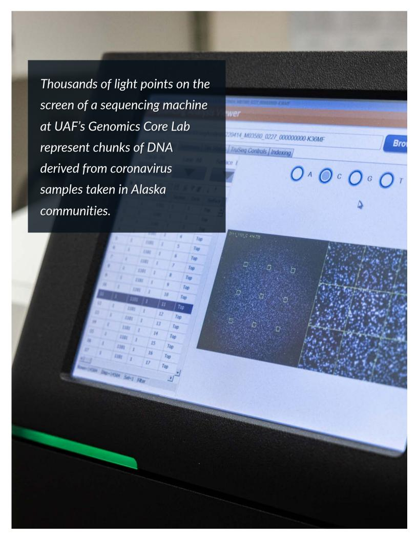
Inside the box, a series of chemicals, called reagents, had washed over that DNA and attached fluorescent molecules to each nucleotide. The specific colors in the fluorescence reflect the presence of adenine, cytosine, guanine or thymine, the four base molecules that all DNA contains, and how they're paired within the nucleotides.
