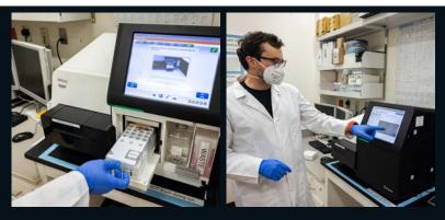
Clockwise from top: Logan Mullen holds a flow cell; Mullen describes information on the screen of the machine that sequences genetic material that he has dropped into a flow cell; Mullen inserts a cassette that contains chemical reagents that attach fluorescent chemicals to nucleotides in the genetic material, giving each type of nucleotide a specific color that can be detected and recorded by the sequencer.
