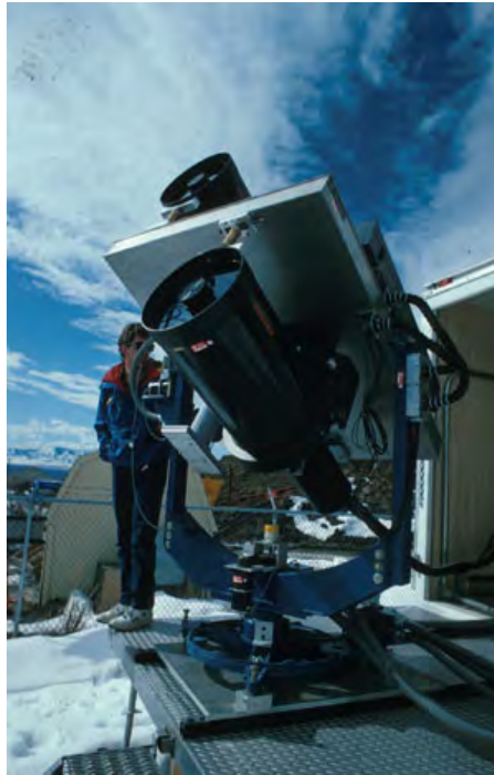
FIG. 2.2. a) Interior view of the FARS site showing the zenith-pointing cloud polarization lidar (CPL) and coaligned midinfrared radiometer beneath the observation skylight, along with some of the computer controller and video systems; b) Photograph of the polarization diversity lidar (PDL) deployed at the FARS for scanning operations on the mobile platforms rear tailgate, depicting the laser transmitter, dual telescope receiver, and safety radar unit dish (from Sassen et al. 2001).
