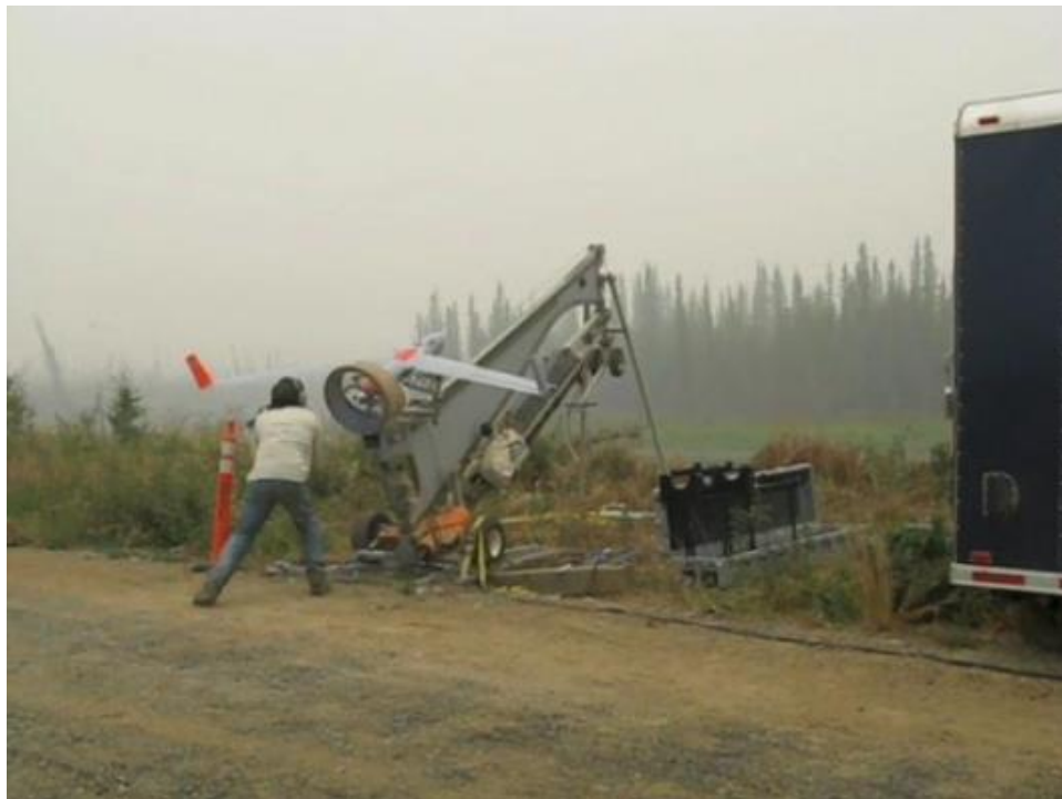
Figure 1.3 ScanEagle being launched into the plume of the Crazy Mt. Complex fires by Circle, AK in August 2009. (Courtesy UAF, 2009)
