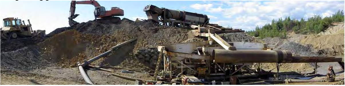
Figure 4 Excavator feeding a trommel. Material then flows into a jig for separation into tailings and concentrates. There is approximately 50,000:1 reduction.
