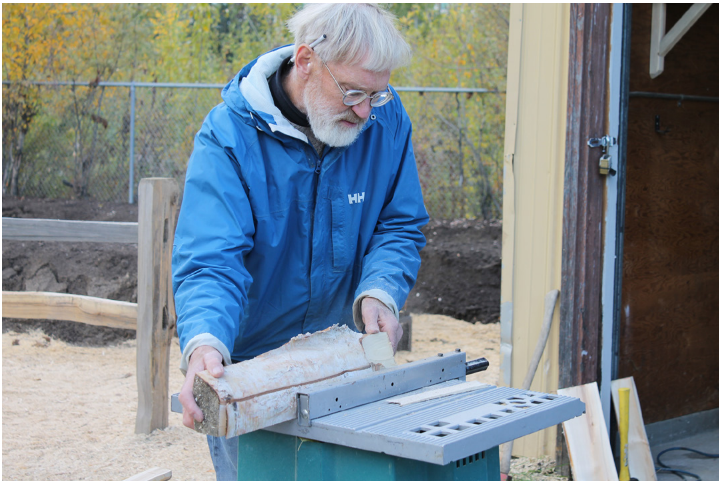
Figure STEAM 21b and c. Birch cuts flitches from round log (above), and then cuts flitches into square stock (below) to be turned.
