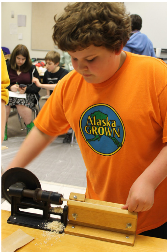
Figure STEAM 22. Seventh-grade student turns square stock into round shaft of knitting needle (above); trims the square end (above right) and sands his finished needle (right). Photo credit: Nancy Tarnai/SNRAS.
