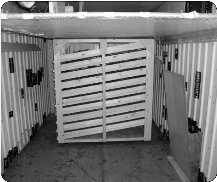
Inside the drying room, showing the drying rack in place. This rack used ten rows of trays, which proved to be too many; in a later design this was reduced to seven rows so that turning the trays would be easier. —PHOTO BY DANNY SLAKEY
