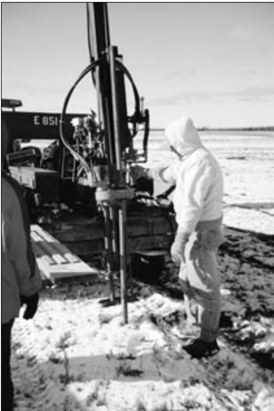
Right: The collected soil samples are bagged, labeled, and taken back to the laboratory in Fairbanks. Each sample is labeled with location information (which treatment plot it came from and the depth at which the sample was taken). Here darleen masiak prepares to bag the deepest depth from a probe sample while Bob Van Veldhuizen holds the probe to keep the sample in until they are ready to place it in the sack.
