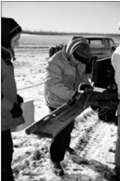
Right and far right: agronomy professor Mingchu Zhang measures and slices a soil sample for each depth within the probe. Together, he and darleen masiak bag the sample.
