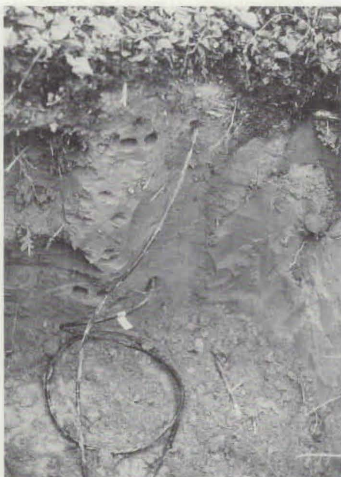
Thermistor soil-temperature probes were positioned at 4- and 10-inch depths at a site in the Yukon Flats.
