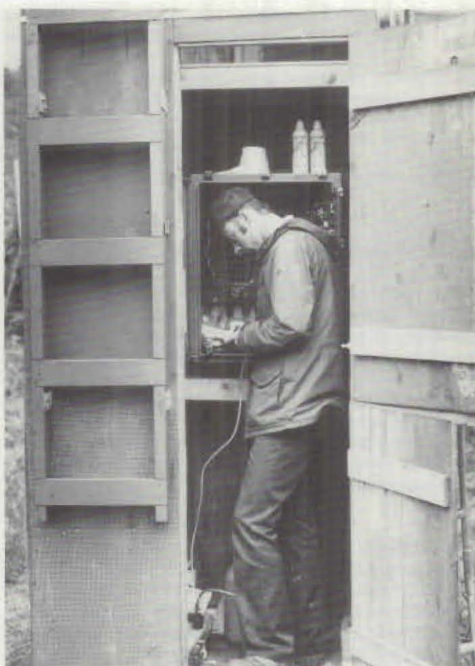
SCS snow survey crew member, Jason Restad, connects cables to the instrument panel of a SNOTEL station. The outside ladder and the two-piece door provide winter access when the snow blocks the lower entrance.
