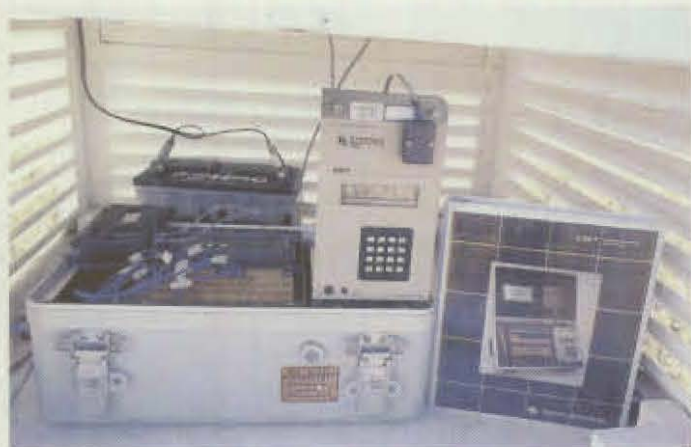
Figure 1. View of the CR7 datalogger installed in conservation tillage research at the UAF Agricultural and Forestry Experiment Station tracts near Delta Junction.
