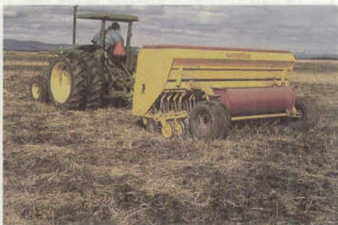
Figure 4. The double-disk, press-wheel drill disturbs the soil only enough to place seed and fertilizer in a slot formed by the disks.
