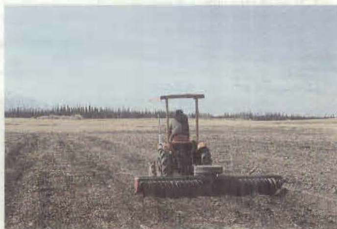
Figure 3. A packer used prior to seeding on plots which are tilled helps firm the seedbed.
