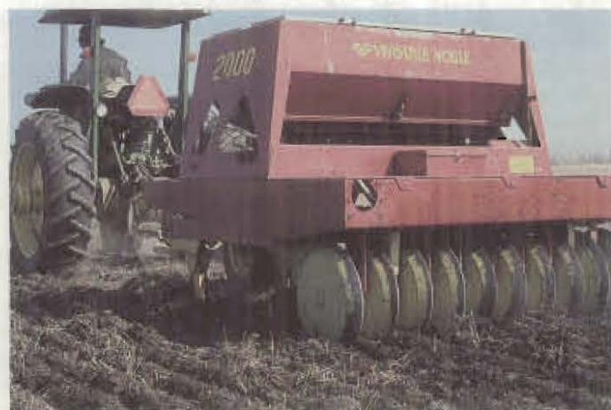
Figure 5. When the hoe drill is used, considerable soil disturbance occurs. Press wheels on the drill, however, ensure good contact between seed and soil.
