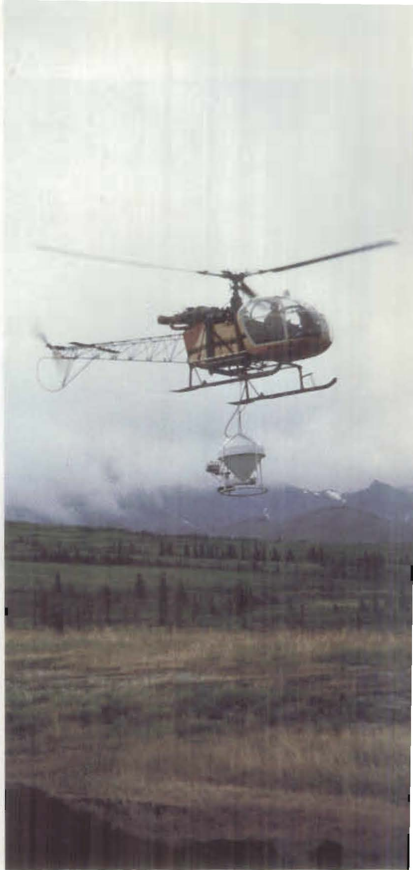
This helicopter is used for fertilizing newly reseeded areas at the Usibelli Coal Mine near Healy, Alaska. The fertilizer spreader, seen suspended from the aircraft, is powered by its own gasoline-fueled engine. At the appropriate time, the pilot opens the spreader and applies a standard, high-nitrogen, granular-pellet fertilizer. Helicopters are also used for the distribution of the mixture of grasses, legumes, and annual mustards used in the revegetation of coal-mine spoils and roadways.
