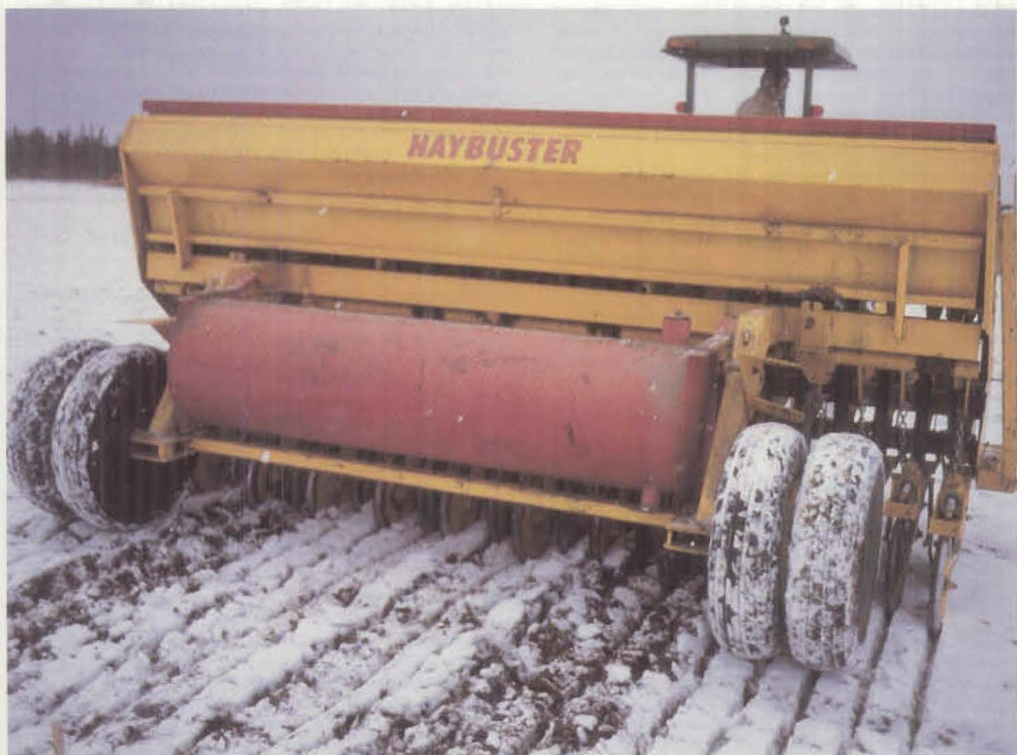
Fall planting in frozen ground can be accomplished with a no-till grain drill such as this Haybuster Microseeder.
