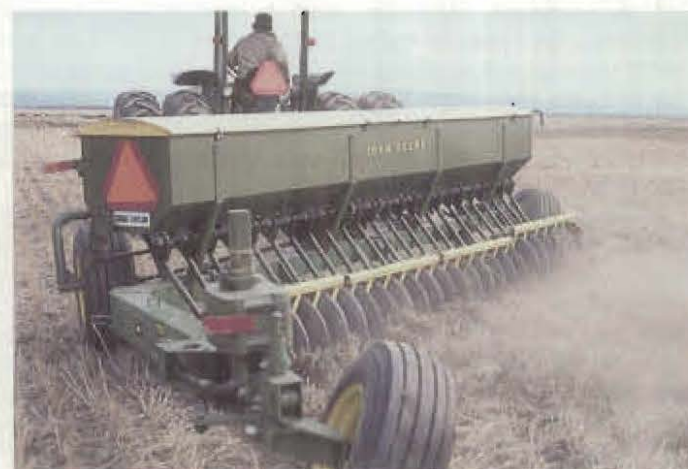
Figure 6. The disk seeder does not place the seed in straight rows. The visual effect is similar to that achieved when broadcast seeding. A packer can be pulled behind the disk or used as a separate implement to ensure a firm seedbed.
