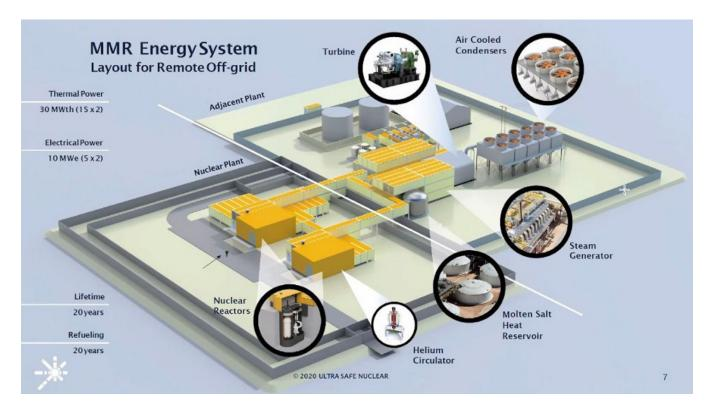
**Figure 2.4.** A proposed layout for the Ultra Safe Nuclear Corporation Micro Modular Reactor Energy System (MMR), which incorporates two reactors each capable of supporting 5 MW of electric power generation. Other configurations are also possible, including a single unit or multiple units. (Image courtesy of USNC)
