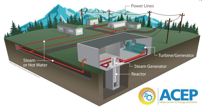
**Figure 2.2.** Conceptual layout of a generic SMR or MNR plant. An SMR or MNR is designed to be delivered to the site with key components (or in some cases the entire system) packaged in self-contained housing that is designed to be placed below grade. Many of these reactors generate steam which is used to generate power. Heat can be delivered via a steam or hot water district heating system.
