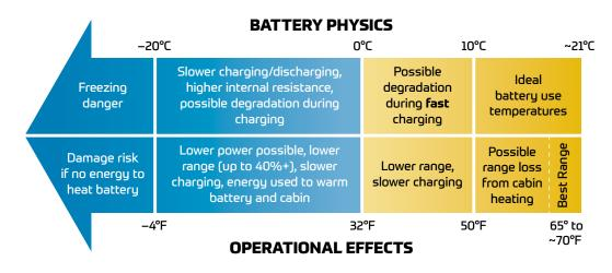
Effects of cold temperatures on batteries and EVs. The top half shows temperature effects on batteries based on physics. The bottom half of the figure shows the operational effects on EV performance. Source: Cold Weather Impacts on EVs, Michelle Wilber, Alaska Center for Energy and Power
