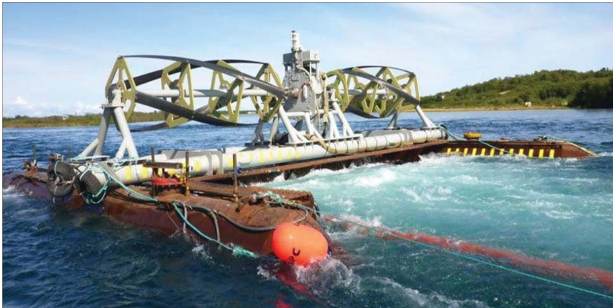
Figure 5. ORPC's cross-flow horizontal axis RivGen system prior to submersion for testing on the Kvichak River near Igiugig, Alaska.(Photo courtesy of ORPC.).
