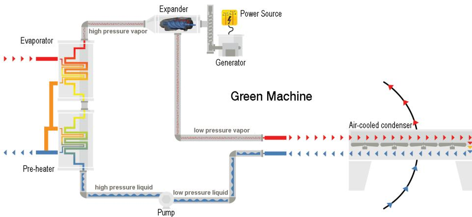
Step 1: Heat is captured by the evaporator and boils the working fluid into pressurized vapor.
