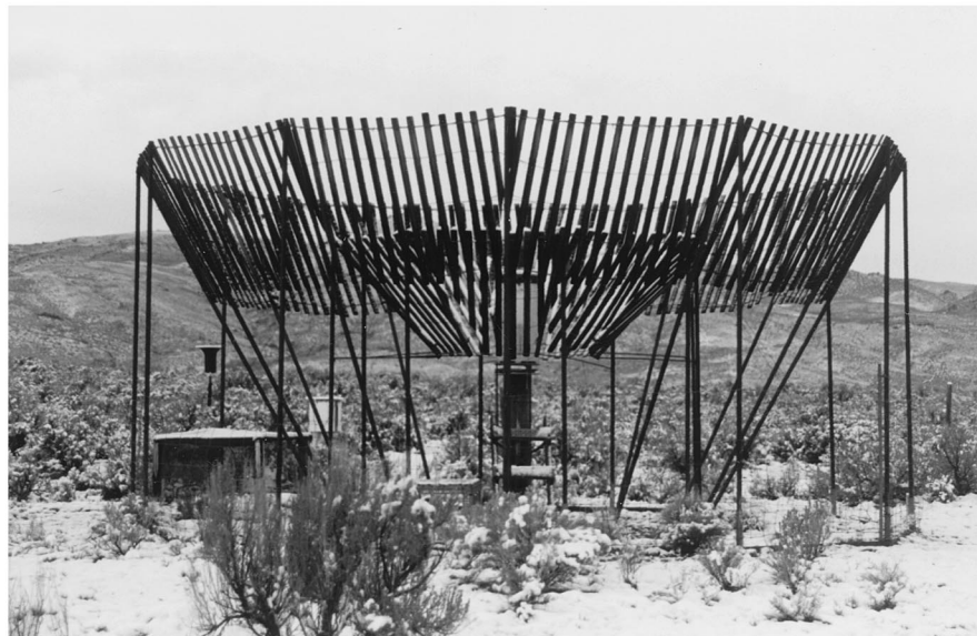
Figure 1. (top) Photos of the World Meteorological Organization (WMO) Double Fence Intercomparison Reference (DFIR) and the (bottom) Wyoming shield.
