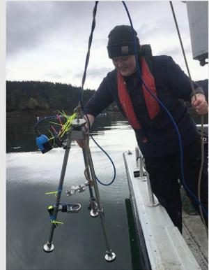
Image 1. Deploying the drop camera.
