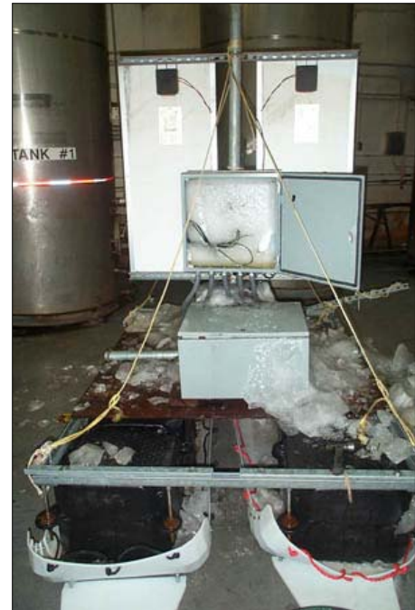
The weather station, minus several layers of ice. Note the remaining ice buildup in the instrument box. Photo by L. Hinzman.
