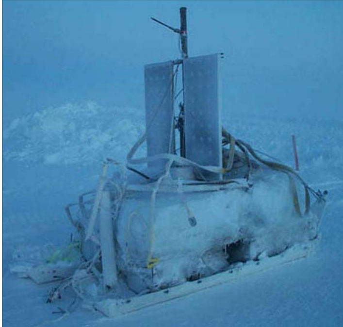
The freed weather station. Dan Miller estimates the "ice cube" weighed 1,000 kg when they pulled it from the lake. Photo by L.Hinzman.
