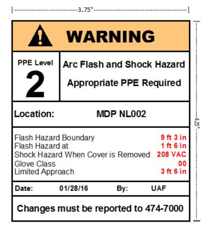
Where UAF is name of company performing Arc Flash and Shock Hazard calculations.
