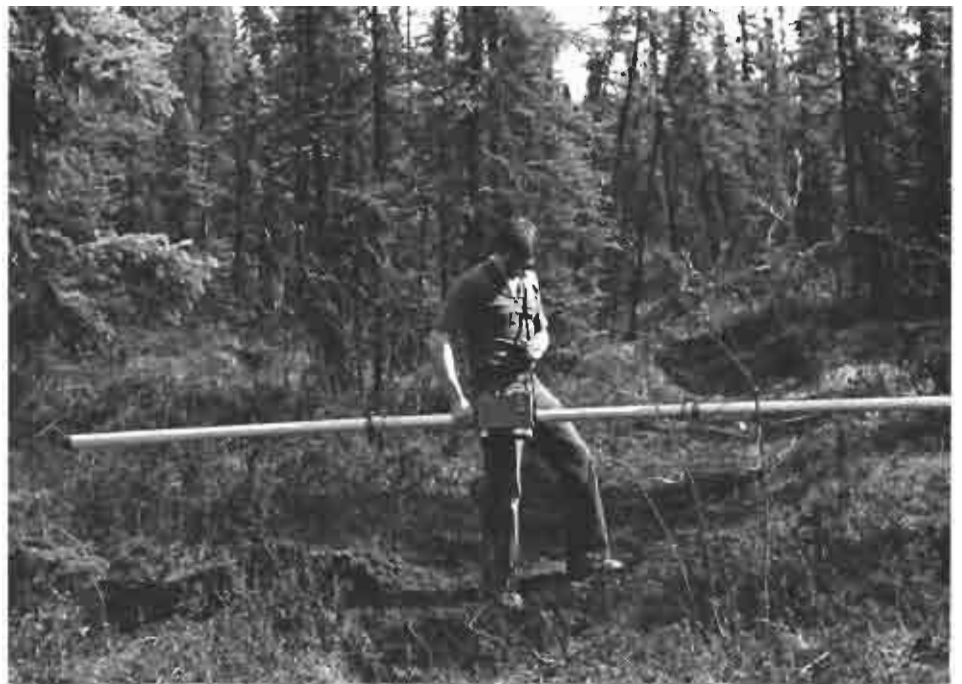
Figure 3. Author Robert McHattie measuring terrain conductivity with the EM-31. Although the 12-foot boom somewhat limits maneuverability in heavy brush, the instrument is lightweight and well balanced.
