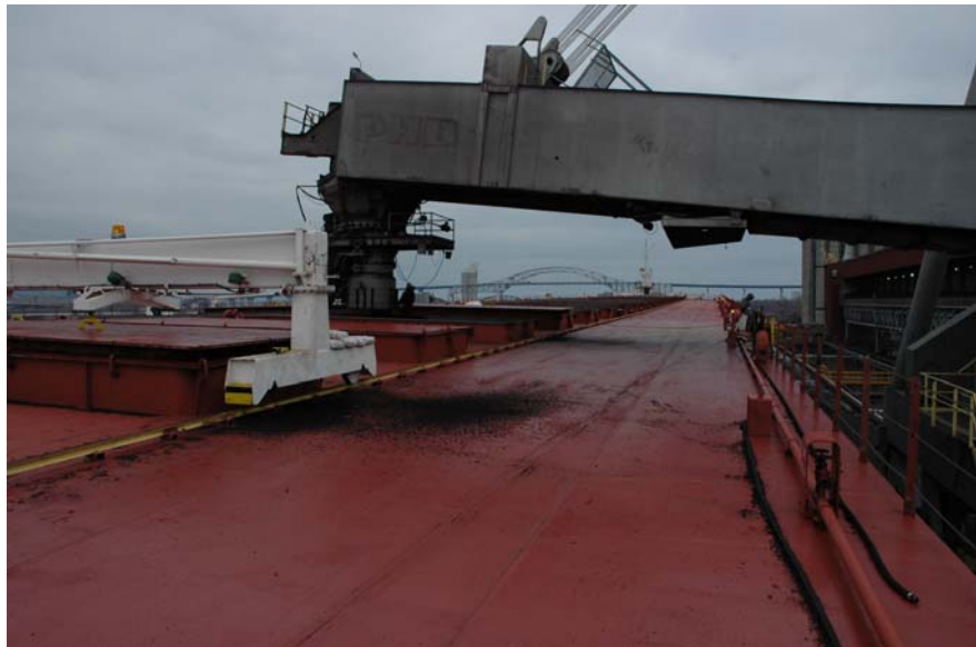
Coal residue, a dry cargo residue, collects on a ship's deck during loading operations.
