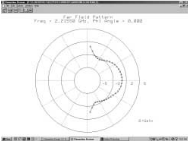
Figure 3.5.2.1: The radiation pattern of the patch antenna
