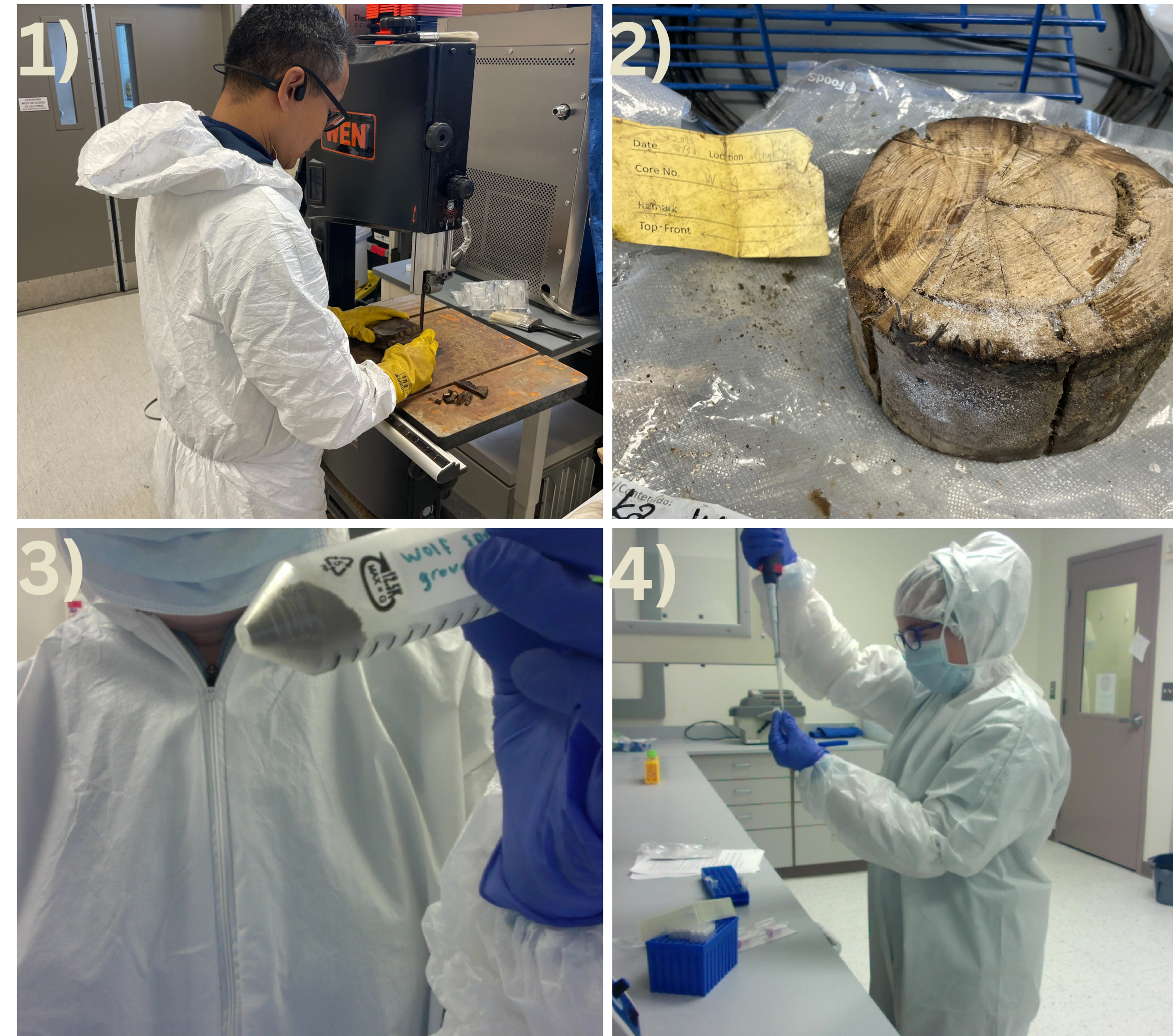
Images: 1) Dr. Go Iwahana using a band saw to subsample one of the 8 samples of ancient Spruce wood. 2) Sample 5 out of 8; the freshest sample of Spruce wood and was used in this extraction. 3) Specimen ground up, ready for extraction. 4) Bree using the DNeasy Plant Mini Kit to extract DNA from the ancient Spruce in the ancient DNA lab at the UA museum. Protective gear is required to avoid contaminating samples with modern DNA.
