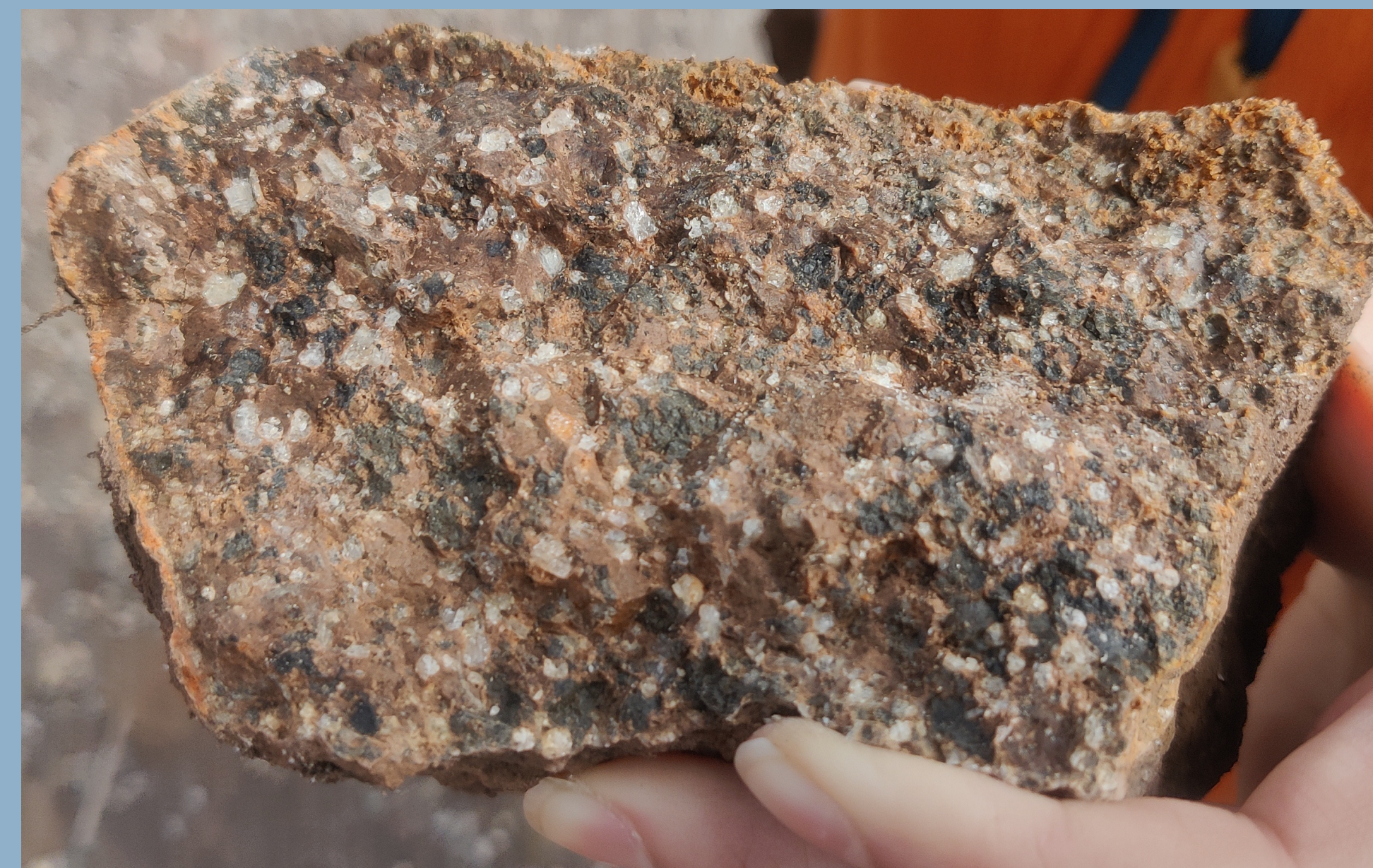
Figure 2: Hand sample of Alder Creek Rhyolite showing large feldspar crystals, which are used as a standard for ^{40}\text{Ar}/^{39}\text{Ar} dating.
