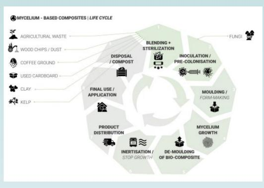
Diagram depicting the life cycle of fungal mycelium bio composites, poster: Material Computation with Myco-materials (Gough et al 2022)
