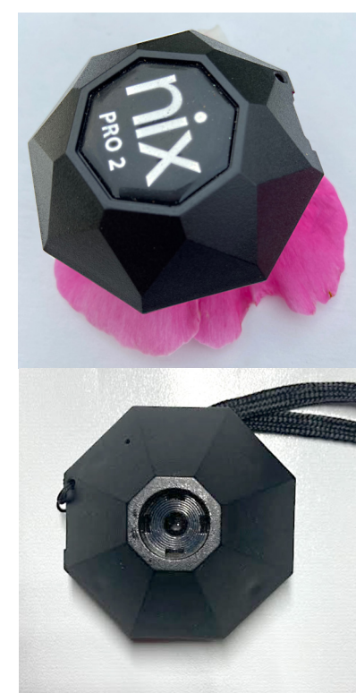
Fig. 1. Top and sensor view of Nix Pro 2® Colorimeter
